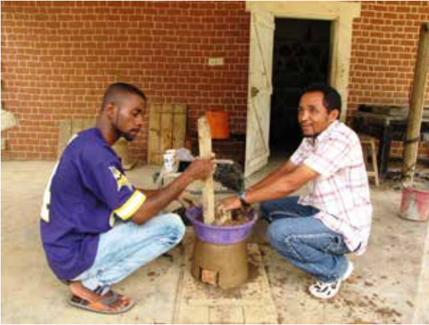
Lanto (on the right) and Razaka making a rocket stove.
