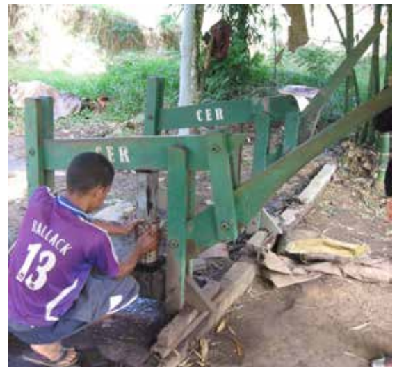
Pressing mechanism for making "green charcoal".
